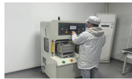
Ingress-Protection (IP) Airtightness Test
