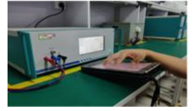
Electrical Fast Transient/Burst Test
